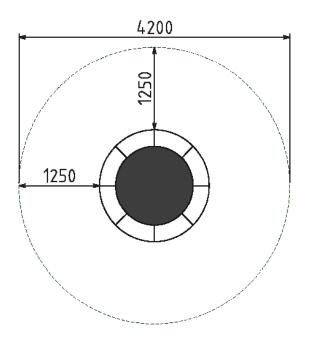
NOTE: A clearance zone of 1500mm is required around the bouncing surface. The safety slab is part of the clearance zone. An additional 1250mm clearance zone must be included. The clearance zone must have a HIC greater or equal to 1000. The safety area above the surface must be
